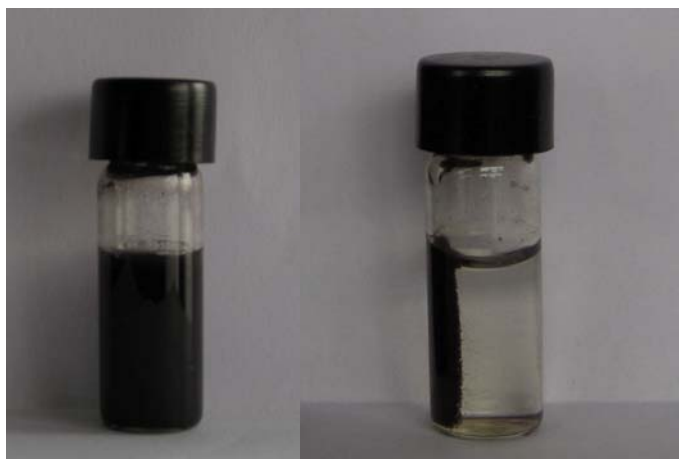
图 4 磁性纳米粒子分散在溶液中（左），外加磁场下粒子被吸引到瓶壁（右） Figure 4 Magnetic nanoparticles dispersed in water (left) and can be drawn from the solution to the sidewall of the vial by a magnetic field (right).
